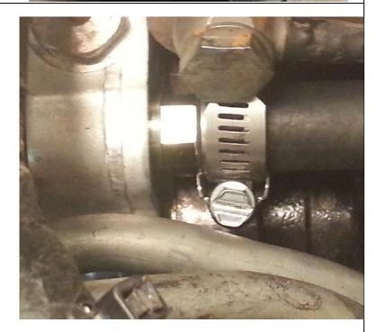
7. If using a BD Flowmax pump. Thread supplied 1/2" barb fitting into the pump inlet and secure with a hose clamp, cut hose to length as necessary.
