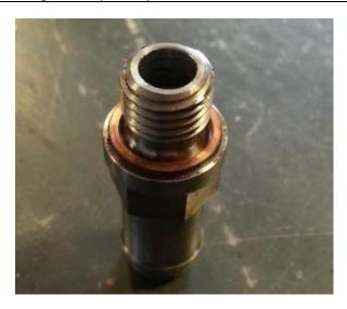
7. Once the washer is switched over, thread the HiFlow fitting into the CP3 inlet. Torque the fitting to 6ft-lb (72in-lb).
