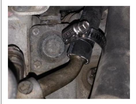
13. Ensure the abrasion sleeve is in the correct position and the hose is secured properly to avoid leaks and chafing.
