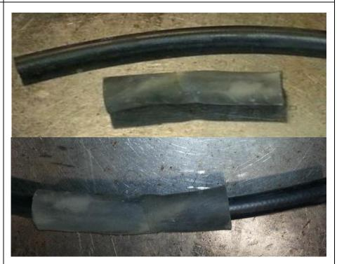
Push the 1/2" hose over the HiFlow barb and secure tightly with a socket.
