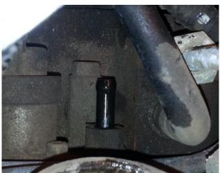
Remove the CP3 inlet fitting and transfer the sealing washer over to the new HiFlow fitting as shown.
