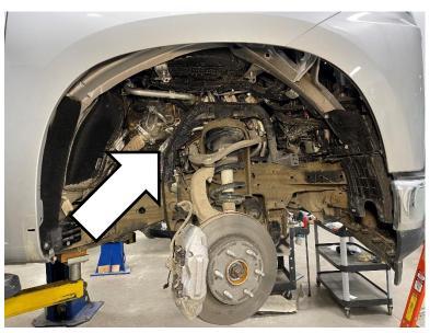
Remove the passenger side wheel, fender liner, and skid plates to get closer to the sensor. The sensor is behind a heat shield near the exhaust that can be unscrewed and moved out of the way as shown:
