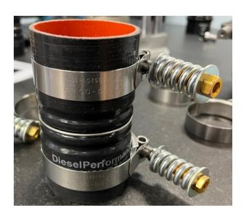
Slide the boots onto the OEM passenger side CAC pipe and reinstall the CAC pipe.
