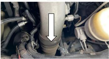
Slide 2x **1405212** clamps onto the **1401563** boot and insert the shorter end of the CAC pipe (**1401564**) into it.
