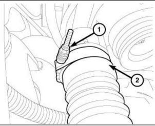
Slide 2x **1405209** clamps onto each of the **1302426** boots as shown.
