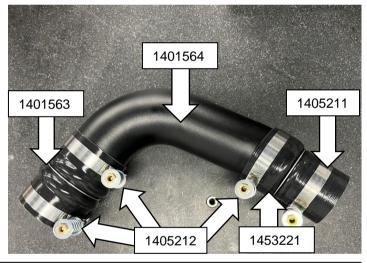
Install the cold-side CAC pipe. Using a ½" socket, tighten the clamps until the springs are fully compressed.
