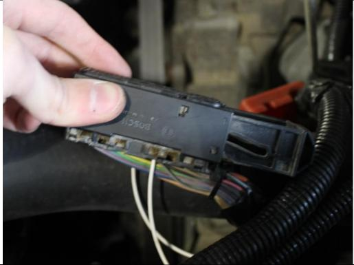
View the connector from the ECM side and ensure the pin is fully seated by comparing to adjacent pins. Lightly tug on the wire to ensure it is fully seated and locked. Reinstall the pink pin retainer back into the connector. If this clip is not easy to insert, one of the pins is not fully seated and may need to be inserted further.
