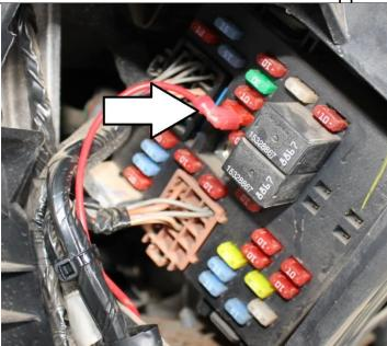
Route the black wire to the head of a bolt below the dash to serve as a ground. Remove the bolt using a 10MM socket and ratchet, install ring terminal and reinstall the bolt.
