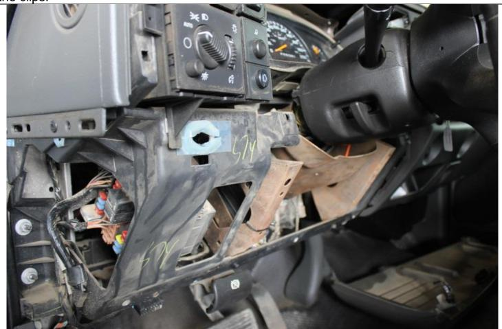
Position toggle switch near the desired location keeping sufficient wire slack. Feed the wires below the dash.
