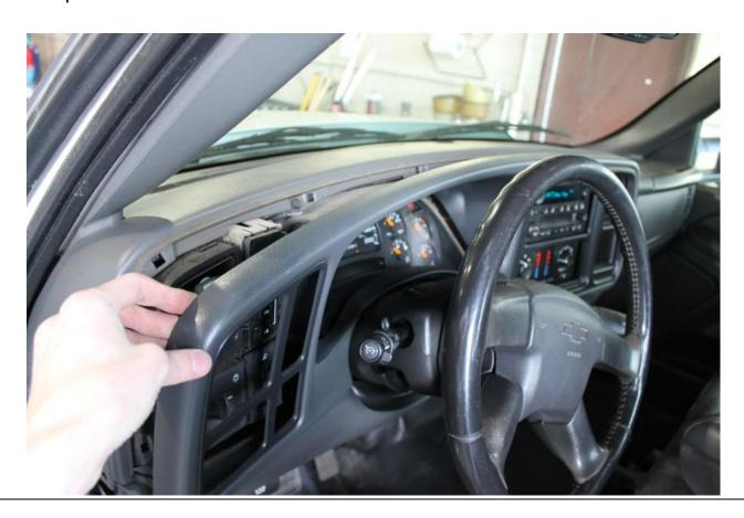
Remove fuse cover from end of dash. Remove knee bolster by removing the two 7mm screws along bottom edge, and then pull knee bolster outwards. Use care not to damage the clips.
