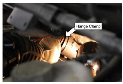
10. Connect the passenger side up pipe to the passenger side exhaust manifold using the supplied hardware. (1900013 & 1900014)
