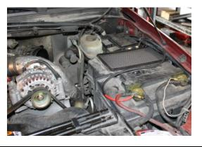
Remove the clamp holding the downpipe to the turbine housing. (7/16" deep socket)
