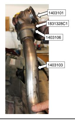
Maneuver the pipe assembly into the vehicle and insert the pin on the collector casting into the turbine housing of the turbo. Install the flange clamp (7/16" socket); tighten enough to allow a bit of movement.
