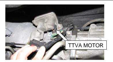
5. Cable tie wiring along transmission across to the frame rail and up the firewall.
