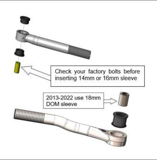
Install the left-hand threaded jam nut (#1302032) on the passenger side track bar section. Thread this all the way to the end. Use a small amount of anti-seize on the threads. The left-hand thread nut will have an <u>arrow</u> on the side face.
