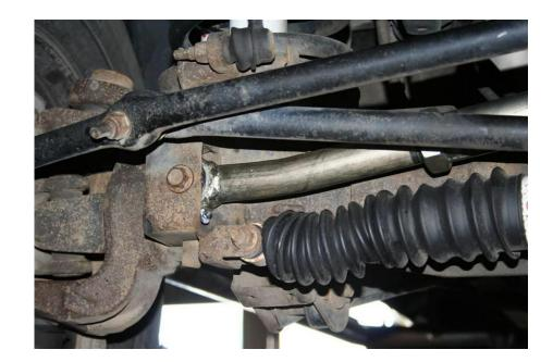
On the driver's side use the 14mm bolt and hardware provided to secure the track bar.
