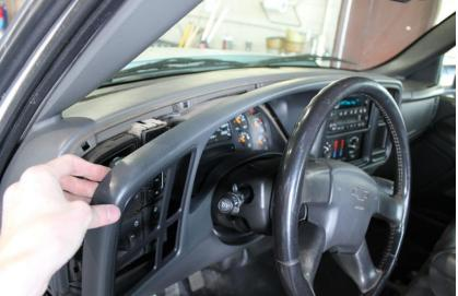
Remove fuse cover from end of dash. Remove knee bolster by removing the two 7mm screws along bottom edge, and then pull knee bolster outwards. Use care not to damage the clips.
