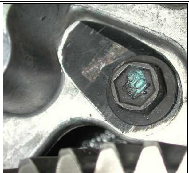
With retainer and bolt installed
