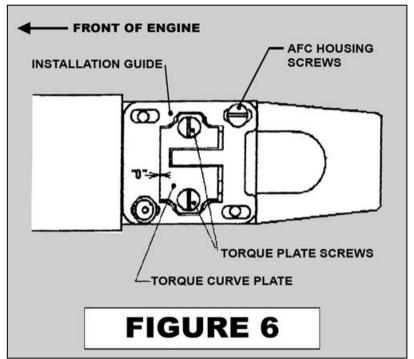
nearly zero clearance between the front of the torque plate and the installation guide.
