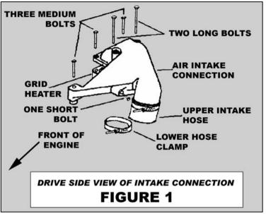
6) Remove the six bolts holding the air intake connection and dipstick tube in place using a 10mm six-point socket. Take note of the bolt locations as they are different lengths and need to be re-installed in the proper location during re-assembly.
