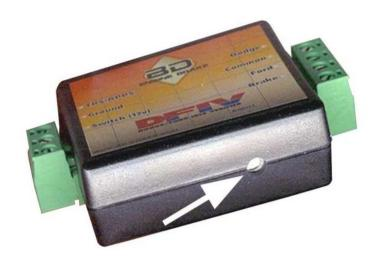
small adjusting screw in the DFIV Module counterclockwise or clockwise until the test light JUST turns on.
