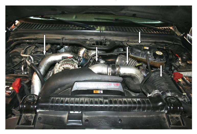
Remove the air cleaner assembly by disconnecting the MAF sensor and Filter Minder device. Then remove the ribbed hose, then the air box. Remove the two (2) 8mm bolts securing the hard tube. Then remove the breather tube from the vent on the driver side rocker cover. (NOTE: Wiggling and pulling out on the tube will help in removal).
