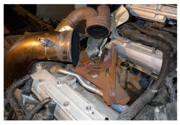
10. Reinstall the turbo charger by reconnecting the connector on the turbo solenoid and clip, the oil feed link, exhaust downpipe, and exhaust feed pipe clamp. Reinstall the three (3) 10mm mounting bolts to hold the turbo in position.
