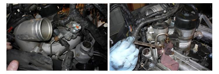
Disconnect the fuel filter wiring connectors and fuel lines then remove fuel filter housing.
