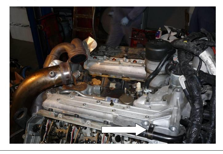
9. Reinstall the oil drain pipe & turbo pedestal mount using four (4) 10mm mounting bolts.
