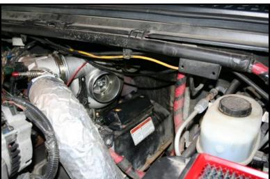
3. Remove two Phillips screws on the top of the driver side valve cover.
