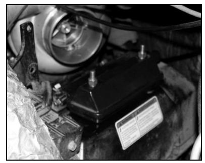
4. Install inlet hose (#1302178) onto breather vent. Use the #32 spring clamp (#1302197) to secure this connection.
