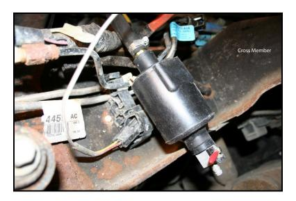
To drain the oil catch can turn the lever to the open position.
