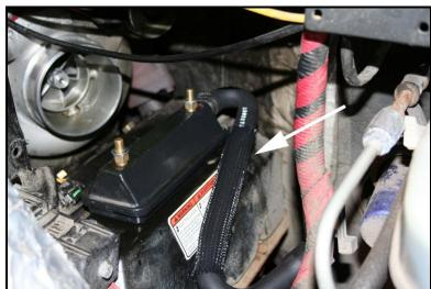
5. Assemble the CCV onto the large stainless bracket with drain hose. You may have to undo the latch on the plastic canister holder and clock the canister to match what is shown in fig 1.1
