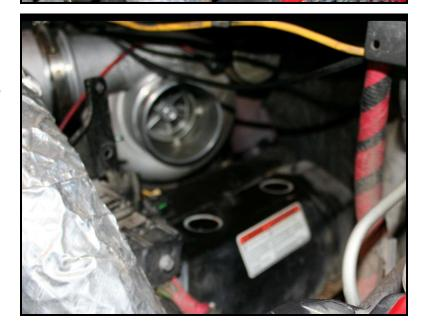
Install new hex bolts with ½ socket. Be sure to install the two O rings over the base of the bolts.
