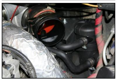
The flow of air should travel out of the valve cover into the top port of the CCV canister. The clean air should leave the lower port of the CCV canister and return into the intake system.
