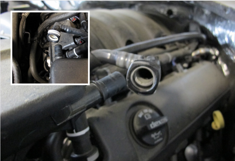
Disconnect the (2) vacuum lines that connect to the air resonator box and valve covers by pushing on the clips and pulling them off from these connections.
