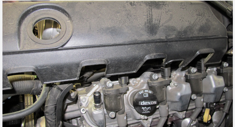
Remove the oil cap then remove the plastic cover from the engine replace oil cap.
