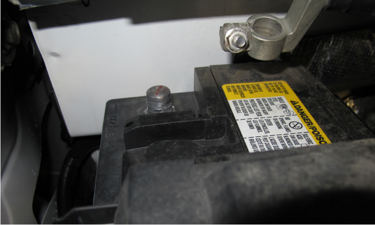
Disconnect the negative battery terminal.
