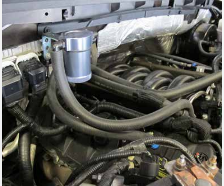
Maintenance empty the oil separator of any oil every oil change or as needed.
