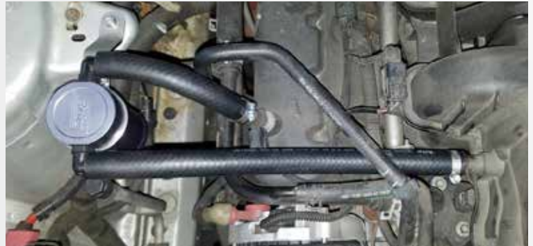
After assembling Oil Separator Kit as shown in pic install it on the vehicle with supplied hardware and clamping down hoses at valve cover/intake manifold connections and strut tower mount.
