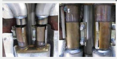
With the BBK head pipe and adapters installed to the BBK full length headers, lift the stock exhaust into place and line it up with the BBK adapter pipes, slide the barrel clamps forward enough to connect the stock exhaust to the BBK head pipe adapters.
