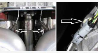
Using a small amount of anti-size on the threads, Install the (2) Oxygen sensors into the BBK Head Pipe Adapters. Run the wiring over the transmission cross member and plug it back into the wiring harness connectors.
