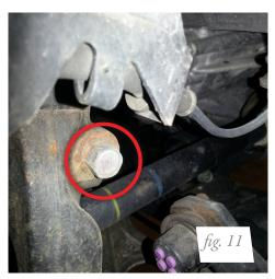
4. Align the fork mount with the lower control arm bushing and insert the previously removed bolt (fig. 12). Tighten the lower bushing bolt snugly, but do not torque at this time. Bolt torque must be done at the desired ride height.
