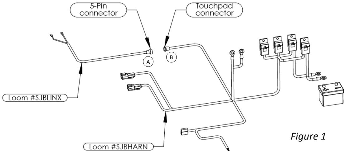
4. Route the #SJBLINX loom and ensure the White and Blue wires reach the LINX controller. Secure the loom with cable ties or tape.
