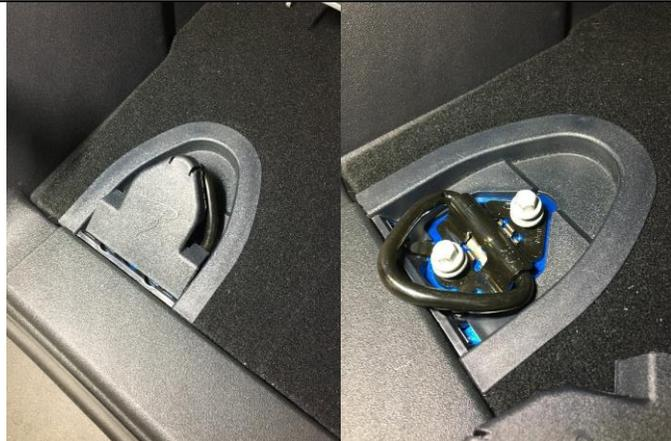
**2.02/- Remove the 2 mounting brackets from the installation kit. Identify Front and rear brackets. Front is shown opposite.**
