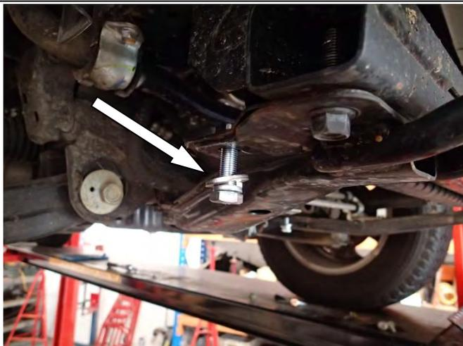
2. As shown in image remove original tow hook bolt and replace with M10 x 35 bolt, spring washer and flat washer. Leave positioned as shown. Repeat for opposite side.
