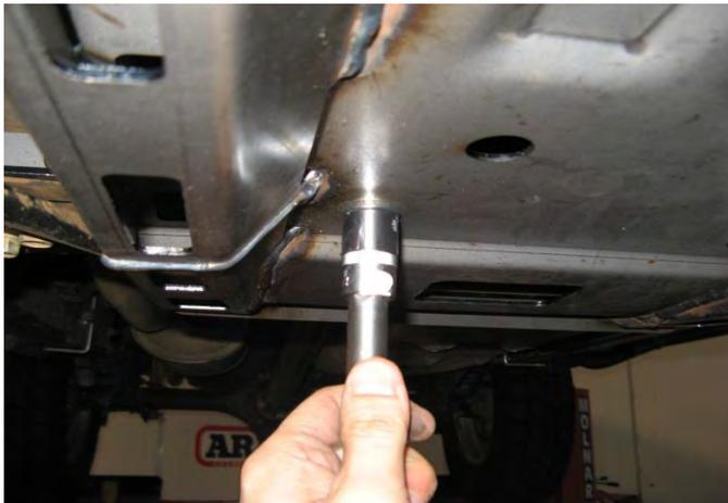
7. Fit transmission UVP and secure to mount bracket using 2 x M10 x 35 bolts, spring washers, flat washers and M10 flange nuts placed on top of bracket. Leave finger tight. Secure to sump UVP using 3 x M8 x 25 bolts, spring washers and flat washers. At this stage tighten all chassis and UVP fasteners as shown by specs below.
