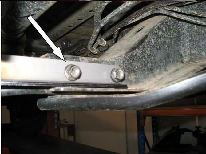
6. Remove nuts only from transmission cross member bolts and fit transmission UVP bracket to front surface. Re-fit nuts and torque.
