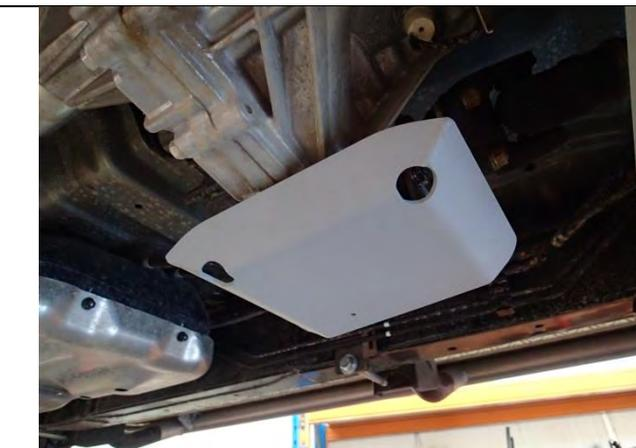
8. Remove O.E panel from transfer case. Fit new guard making sure the return lip is facing the centre of the vehicle. Secure using 4 x M8 x 20 bolts, spring washers and flat washers. Tighten all bolts.
