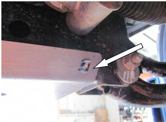
1. Remove original stone shields from vehicle. Insert 3 x M8 cage nuts to rear of supplied front panel as shown.
