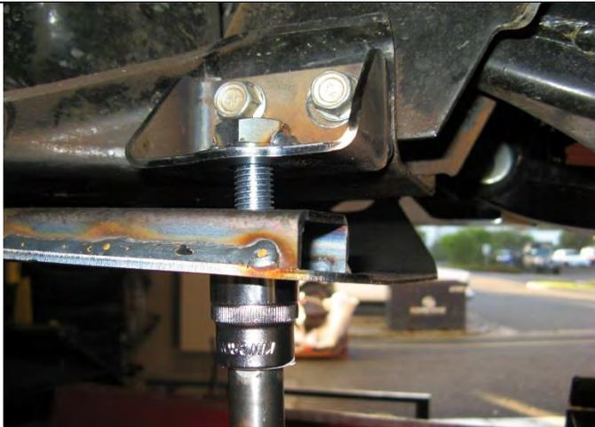
5. Place 3 x M8 cage nuts in rear of sump UVP. Secure sump UVP to chassis brackets using 2 x M12 x 35 bolts, spring washers and flat washers leaving finger tight. Secure front of sump UVP to front UVP using 3 x M8 x 25 bolts, spring washers and flat washers leaving finger tight.
