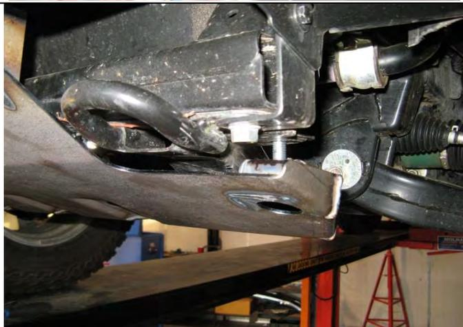
3. Fit front panel as shown by hanging on bolts fitted in step 2. Tighten bolts up slightly to minimise gap but leave loose. Secure rear of front panel to chassis using 2 x M10 x 35 bolts, spring washers and flat washers. Secure front using 3 x M10 x 35 bolts, spring washers and flat washers. Leave fasteners finger tight.
