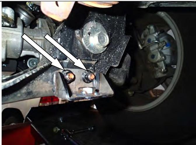
4. Support front suspension cross member using jack or similar. Remove outer two bolts and fit sump UVP brackets to rear face as shown. Do one side at a time. Leave bolts finger tight.
