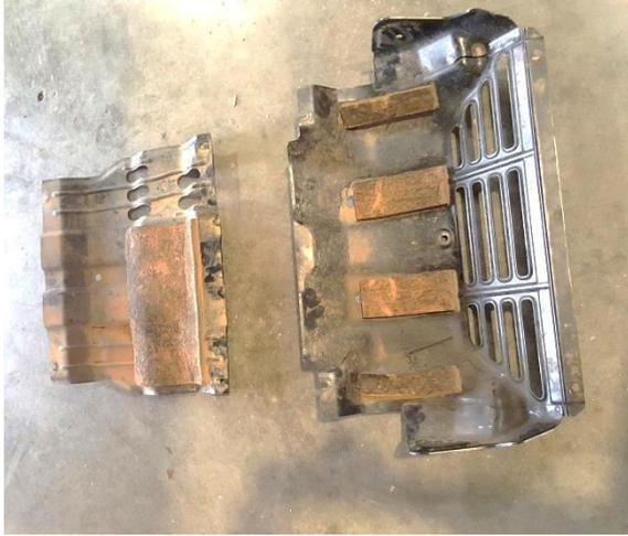
1. Remove OEM panels (front splash panel & diff panel) from vehicle – 6 bolts.
