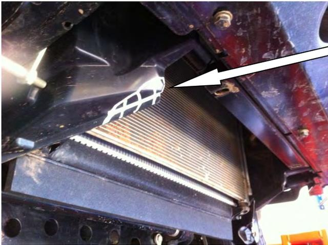
2. Trim plastic air dam using an air saw / multi tool.
