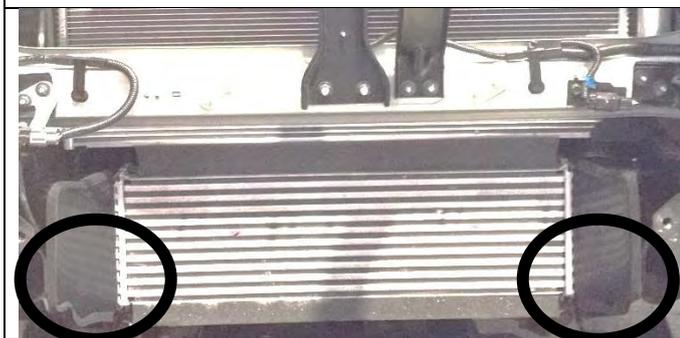
10. Trim lower section of air deflectors located on each end of intercooler by an even 10mm.
