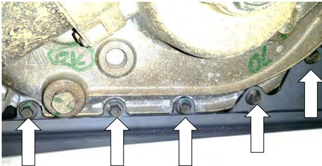
18. Remove 5x fasteners in lower section of transfer case.
