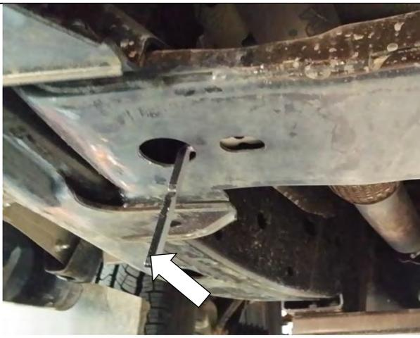
**Note:** Feed nut plates through slot openings located on underside of rear cross member.
