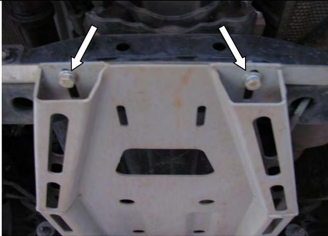
12. Secure rear of panel to bracket using two M8 x 25mm bolts, spring washers, flat washers and M8 flange nuts. Tighten all panel bolts when done including front stone shield bolts.
