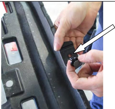
2. **VEHICLES WITHOUT ARB BULLBAR:** Refit OE lower air deflector by first removing the scrivet located in the centre hole.
