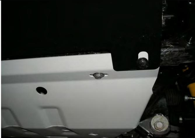
5. Place panel onto chassis making sure it sits under the bullbar stone shield as shown. Secure to vehicle using original hardware removed earlier leaving all bolts finger tight. Secure stone tray to UVP using M6 bolts removed in step 1.
