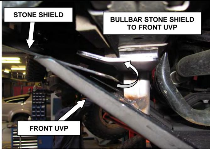
4. Lift front panel into position while placing (if fitted) the bullbar stone shield between the panel and front mounting bracket. Secure panel to chassis using original fasteners and stone shield with M6 bolts removed in step 1
