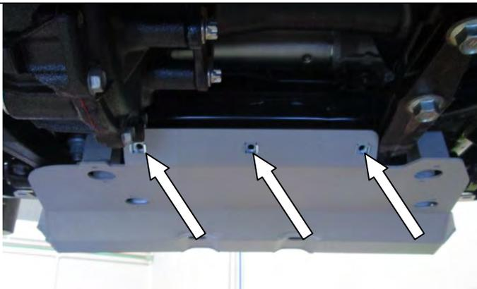
6. Place 3x M8 cage nuts in rear face of front panel.
