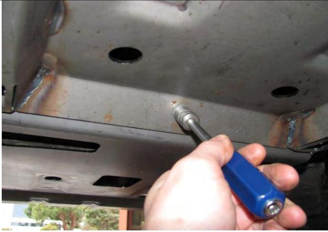
11. Lift transmission panel into place and secure to centre panel using three M8 x 25mm bolts, spring washers, flat washers and flange nuts (outer holes only). Leave finger tight.
