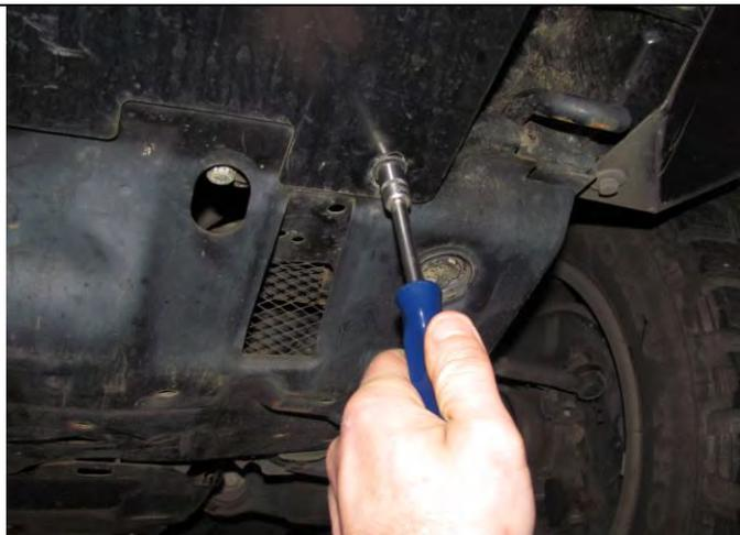
1. **ALL VEHICLES:** Remove O.E panels from vehicle and retain bolts. If fitted with a bullbar remove and retain two lower M6 bolts and loosen off the top four M6 bolts on the bullbar stone shield.
