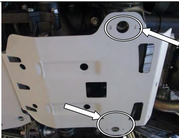
7. Place centre panel on vehicle as shown and secure rear outer mounts to chassis using original fasteners. Leave finger tight.
