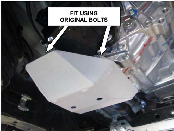
13. Remove original transfer case shield and retain bolts. Fit transfer panel as shown using original bolts.
