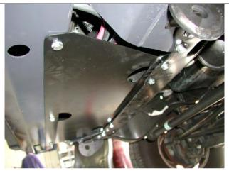
24. Bolt the air deflector to the underside of the bar and chassis cross member using M8 bolts, M8 flat washers and M8 spring washers.
