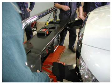
19. Using two people, three if a winch is fitted, position the bar assembly on the vehicle mounts. Make sure the deflector is held down for the bar to be pushed back.
