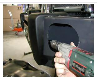
21. The bar must be pin bolted to the mount brackets. Using a drill and 10mm drill bit, drill through the upper and lower Ø10mm holes located in the mount brackets.
