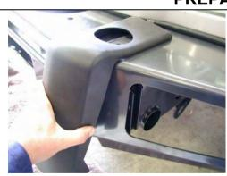
Insert the side buffers through the holes and fix using the M6 flange nuts. (LH Shown).
