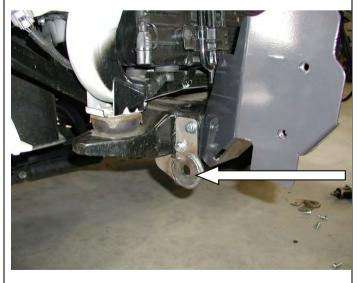
4. Fasten the mount brackets and tow hooks to the end of the chassis rails using M10 bolts, M10 flat washers and M10 spring washers.
