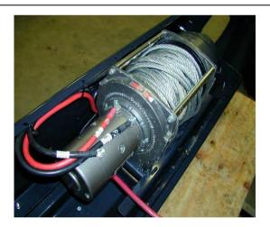
17. Position the winch inside the bar cradle with the clutch handle positioned on the driver's side. Cable spools from the bottom. Bolt in position with the roller fair lead in place.
