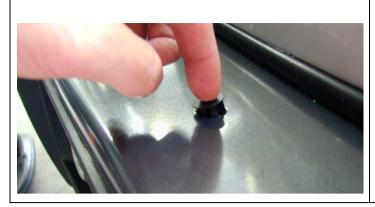
27. There are two Ø16 holes located on the top face of the bar. If no CB aerials are fitted the holes can be covered with the plastic plugs provided in the fitting kit.
