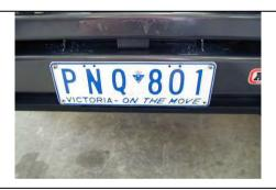
13. Bolt the number plate through the top holes using M6 X 16mm bolts and M6 flange nuts. If desired the double sided tape can be used down the sides of the number plate.
