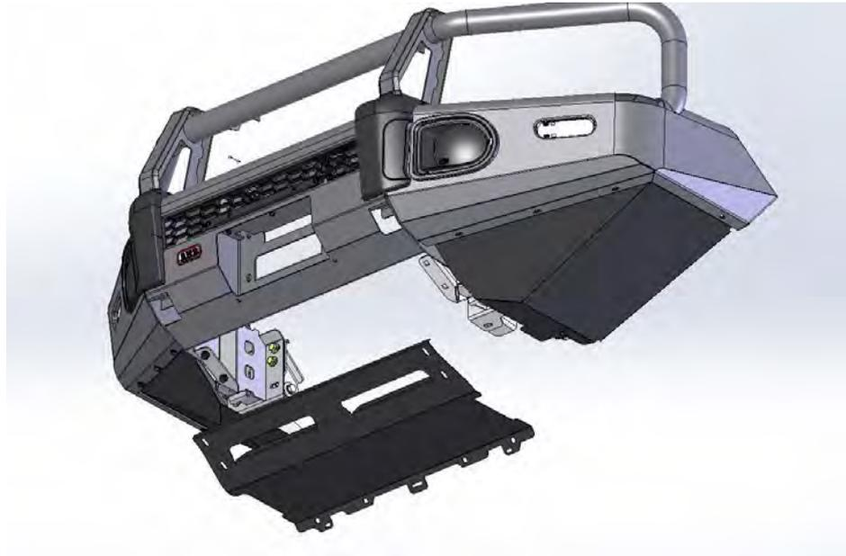
2. Fit 4 x M6 cage nuts to Cover Panel.
