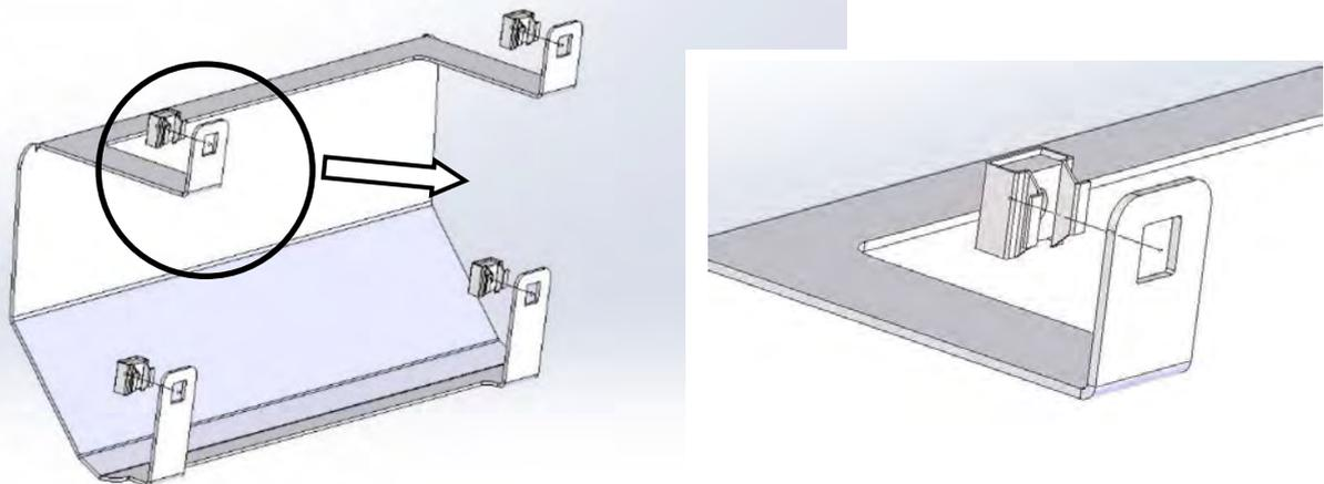
3. Fasten Cover Panel to bull bar using 4 x M6 bolts, 4 x M6 flat washers.
