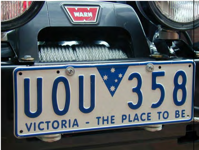
Bolt license plate to bracket using M6 hardware supplied.
