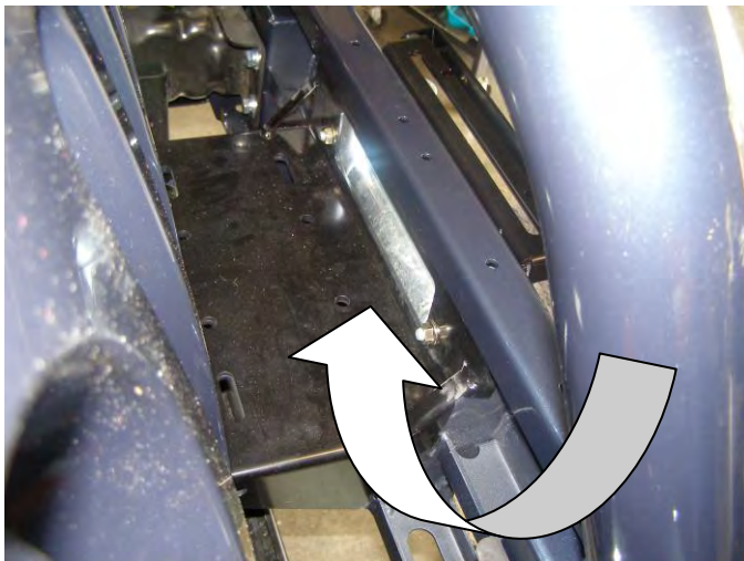
WINCH MOUNTING PLATFORM
