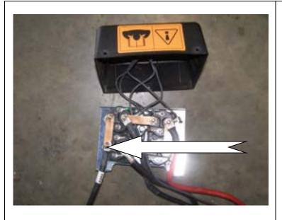
38.To fit control box to bar, you must change the arrowed lead (yellow tagged) in photo with the longer lead that is supplied in fitting kit. When all is fitted, screw plastic cover back onto control box.
