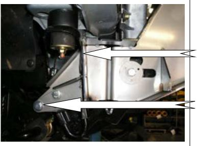
27. With the side and rear bolts fitted, fit the most rearward bolts to each side of the vehicle. Tighten all six bolts firmly.
