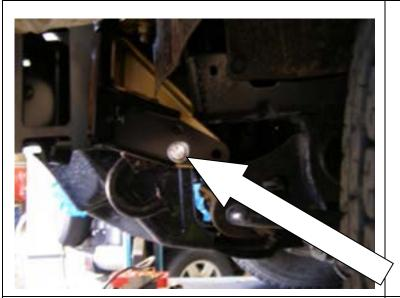
25.LHS side has a hole only, where a 10mm x 30mm 1.5 SEMS bolt is fitted and secured by a 10mm flange nut. FINGER TIGHTEN
