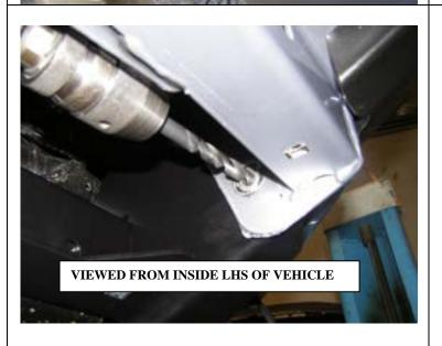
52. When all the six bolts have been tighten firmly, using the lower holes from inside the bar as a template, drill through the impact absorber bracket using a 10mm drill bit and fasten with a 10mm SEMS bolt and a 10mm flange nut.
