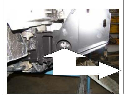
22. Fit impact absorber mounting assembly to vehicle chassis.
