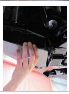
65.Refit the fender liner to the vehicle. Press the fender liner up to the wing under panels and using a Philips screw driver or similar locate and puncture holes large enough to accommodate M6 bolts coincident with the four cage nuts in the wing under panels.
