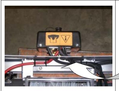
46.Fit rubber grommets into round holes in top of bar, then fit control box to control box bracket and pass cables through rubber grommet.
