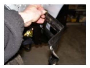
**5.** Remove flare/bumper bracket from vehicle.
