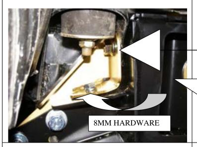
31.Lastly, fit M8 x 20mm bolt, spring washer, flat washer and 8mm flange nut to mounting assembly and tighten firmly.
