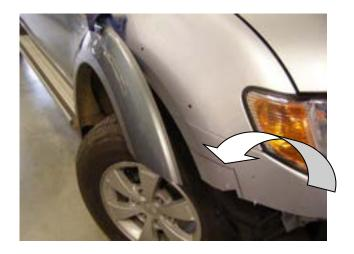
18.Once again lift flare away from guard and cut out marked section.
