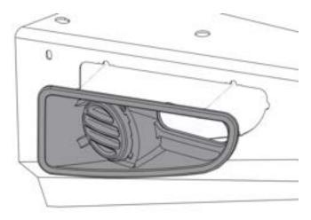
55.Assemble and install combination light surrounds (p/n 3163015) as per instructions no. 3786421 supplied with surround kit. Note: Optional fog lamps can be installed at this point as per fitting instruction no. 3783315 supplied with fog lamp kit no. 6821201.
