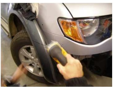
14. Lift flare away from vehicle, and cut along the drawn line, follow the same procedure on the other side.
