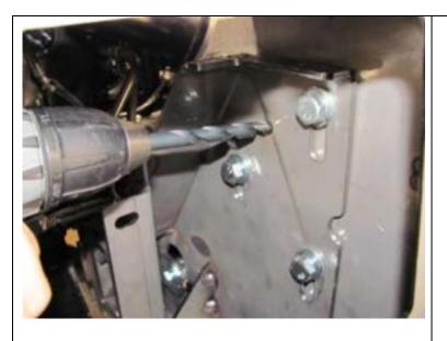
53. Now using the fog light opening as access drill a 10mm hole in the top of the bars upright using the hole in the impact absorbers mounting blade as a template, the pin using M10 SEMS bolt and flange nut, tighten bolt to specified torque.
