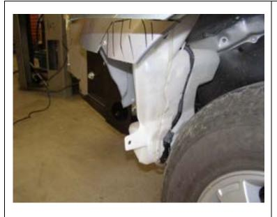
20. When you are about to cut the LHS of vehicle, you must temporarily remove the washer bottle to enable to cut the lower section of the guard panel. Refit flare and washer bottle after cutting.
