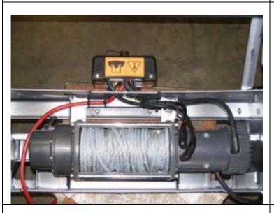
47. Fit all 3 cables to their correct terminals and tighten. Refer to Warn installation instruction when wiring up winch. Fit plastic boots over terminals. Cable tie cables to bar as per photo to clear of all moving parts.
