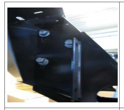
49. With the help of a friend, lift bar in between impact mounting bracket and align slots on mounting bracket to the slots on the side of bar. Secure using M12 x 1.75 x 35 coarse pitch bolts, M12 spring, M12 flat washers and M12 flange nuts. At this stage do not over tighten the bolts to allow for bar adjustment.
