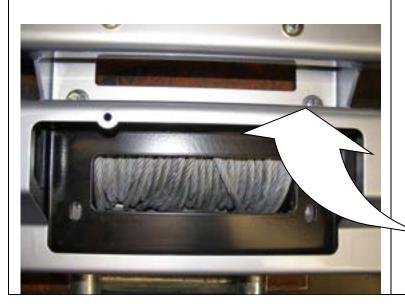
40.Lower bar down over winch, line up top holes first and secure using 3/8" hardware (1 ½"" x 3/8"bolts) flat and spring washers. (finger tighten only)
