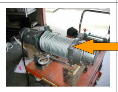
39.To fit winch into bar you must pack winch up on a bench to enable you to lower bar down on winch, then fit four 3/8 " square nuts into winch lugs.
