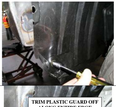
66. Push the fender liner past the wing return and secure the fender liner mounting points using M6 hardware (4 per side).
