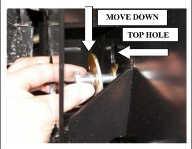
26.Using M10 x 50 x 1.25 mm bolt, 10mm spring washer, large flat washer and packer, feed into top hole and move down and screw bolt into captive nut in chassis.
