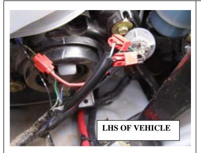
56.Pull indicator loom up into engine bay to scotch lock wiring onto vehicle indicator/clearance lamps
