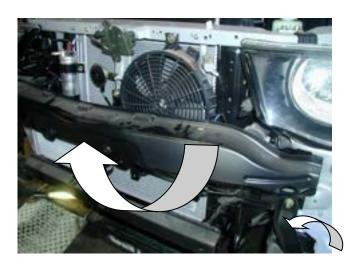
6. Remove cross member and mounting brackets from vehicle.
