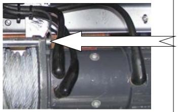
**48.Fit ground wire under winch tie rod.** ( See Photo )
