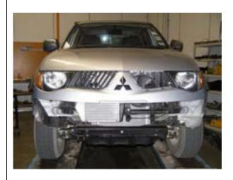
21.At this stage the vehicle is ready to fit impact absorb mounting assembly.
