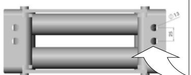
41.Drill two new 13mm holes in the roller fairlead provided in the kit, as shown on the adjacent picture.
