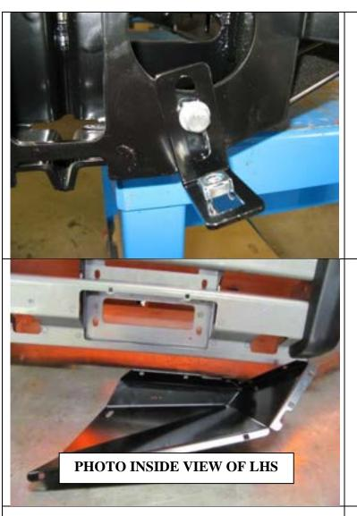
59.At this stage loosely fit the adjustable wing under panel bracket to the mount assembly.
