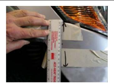
8. At this stage draw a point 120mm down from panel line on each side of vehicle and 20mm in the centre.
