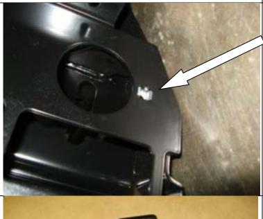
57. The next step is to fit the wing under panels, firstly M8 cage nuts must be fit to the mount assembly as shown.
