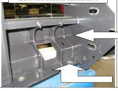
33. The next step is to fit the buffers to the bar using 6mm flange nuts, 6 per side. ( DO NOT OVER TIGHTEN )
