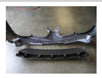
7. With the bumper removed, you must remove lower grille section and fog light aperture rear panels, then refit bumper to vehicle.
