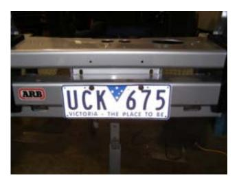
68.If you are not having a winch fitted to the bar, fit plastic grommets into the round holes and secure using black pan head screws to secure number plate to bar as per photo.
