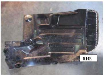
64.Remove plastic inner guards and cut along marked line.
