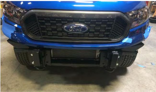
19. Loosely fasten together mounts and reinforcement brackets to front face of chassis using 8x M12 fastener sets.
