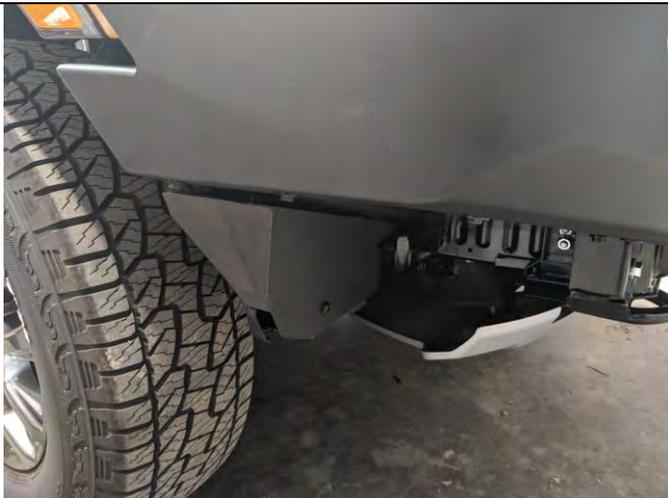
81. Fasten panel onto wheel intrusion bar using M8 hardware supplied in 3540310 and retighten factory M12 bolt.
