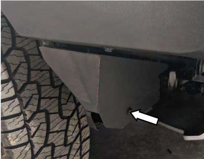
78. Position panel onto intrusion beam as shown and mark hole centre from infill panel onto wheel intrusion bar.
