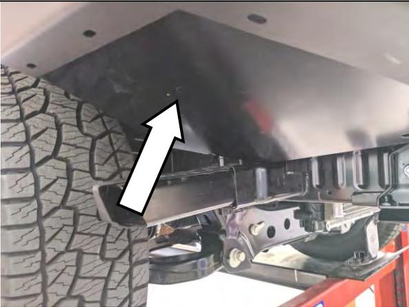
68. Fit the RH under wing panel to the RH wing as shown and attach using 5 x M6 x 20 hex bolts and 5 x M6 flat washers.
