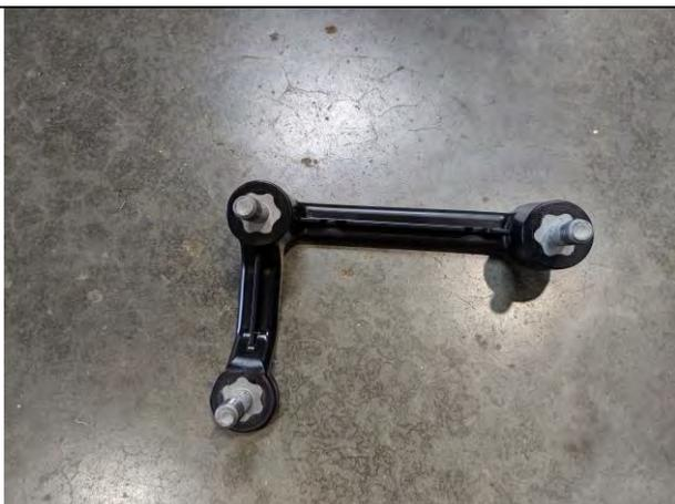
5. Remove captive bolt assembly from each side of the chassis rail.
