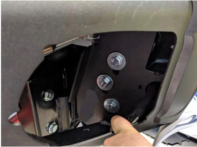
55. Attach the bar to the mount bracket using 3 x M12 x 35 bolts and 3 large diameter M12 flat washers, into the nut plates which are placed inside the box upright sections of the mount bracket. **Leave loose at this stage.**
