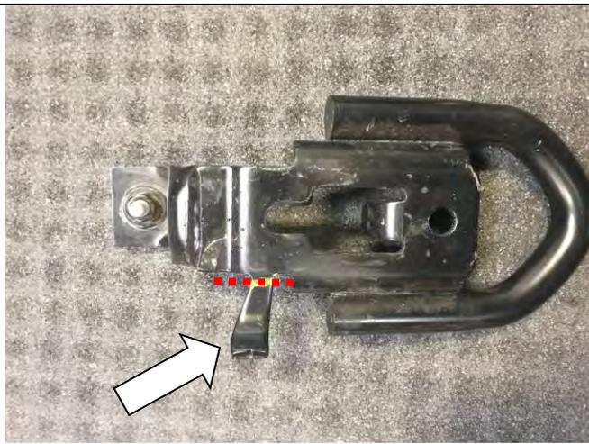
6. Mark line onto tow hook as shown and cut tab off using an angle grinder with cutting disc.
