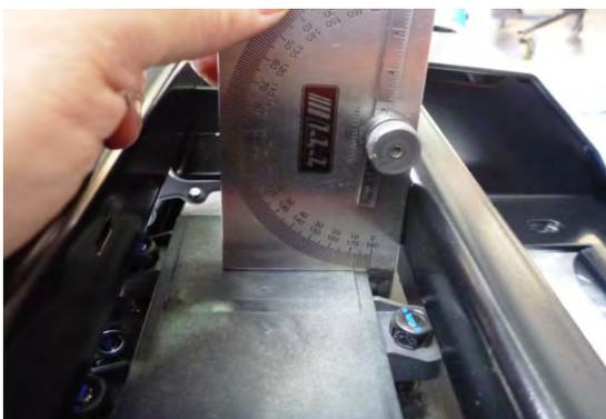
27. Use a square edge to check that the radar front faces are perpendicular to the inside faces of the Upper and Lower Pan at the front of the bar. Make any adjustments if necessary.
