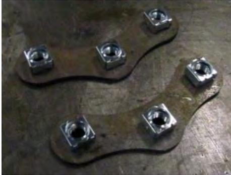
25. Fit 3 x M12 cage nuts to each of the cage nut plates as shown.
