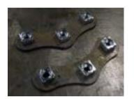
104. Fit 3 x M12 cage nuts to each of the cage nut plates as shown and set aside.
