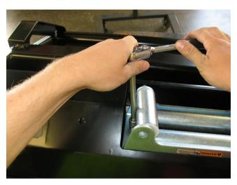
51. Fit the roller fair lead, pull only the end of the cable through and adjust the position of winch then bolt up securely. Use the 1 ½" long bolts in the top and 1 ¾"in the lower set through the RFL.
