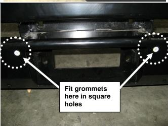
59. Fit grommets to holes in front of pan for number plate mounting
