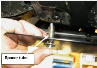
77. Fit stone tray using 4 x M6 bolts and washer sets at front under bull bar and 2 x M6 x 40 bolts, washers and 18mm long tube spacers at two locations into existing sump guard front section as shown.
