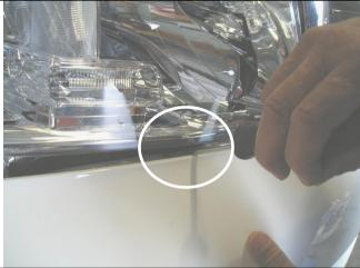
20. Push bumper down immediately below headlamp to gain access with a small flat blade screwdriver and release holding tab.
