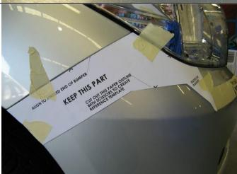
14. Apply template to outer corner of RHS bumper as shown aligning accurately to features such as the lower line of headlamp and end of bumper. Tape in position
