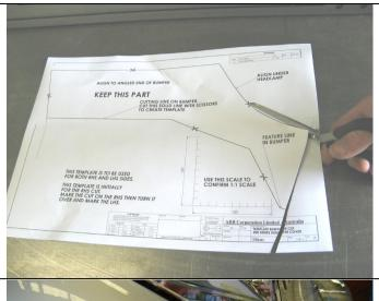
13. Cut A3 paper template along identified cutting line.
