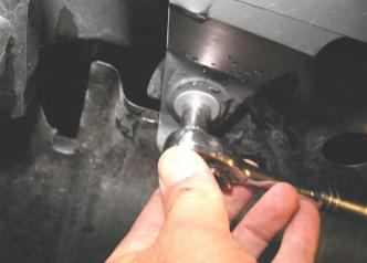
6. Remove lower bumper retaining screws.
