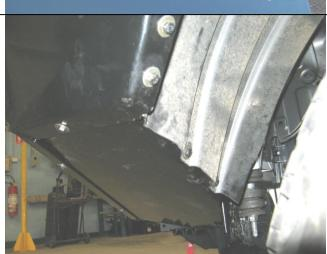
81. Fit 5 x M6 cage nuts to each wing splash panel as shown on *inside* faces.
