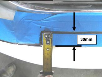
10. Mark out centre cut area of bumper as shown, 740mm wide x 30mm back from feature edge.
