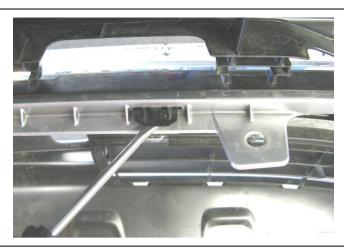
24. Remove grille from bumper cover by releasing plastic tabs as shown
