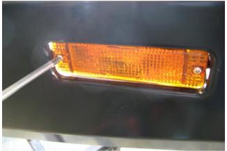
57. Fit the indicators into the recesses both sides of the bull bar as shown, using supplied installation instructions with light kit.
