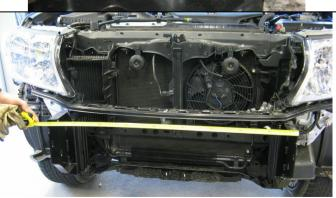
65. Tap the outer flange of the mount brackets until they are hard up against the tow hook mount area. Nip up the lowest outboard nut on each bracket. Brackets should be about 935mm apart
