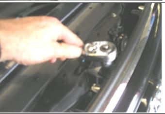
8. Remove retaining screws from top of grille
