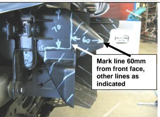
32. Mark the lower section of the air scoop for the power steering radiator as shown. This is for trimming to clear the mount brackets.
