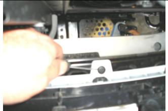
21. Remove plastic plugs securing upper bumper tabs to cross member.
