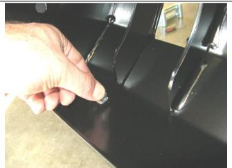
58. Fit 4 x M6 cage nuts to bottom inside face of lower pan in square holes as shown.
