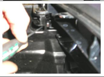
22. Release top of grille. It is retained by 2 x push in spring clips, located at the outer top sections below the bolt position.
