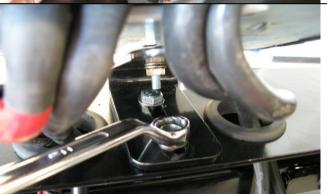
45. Using M8 fasteners fit control box mounting bracket to pan
