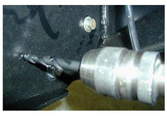
73. Using the M10 pilot holes in mount brackets (located up 175mm from bottom face of bar), drill pinning hole through uprights on bull bar. Fit M10 screw, washer set and flange nut and do up tight.
