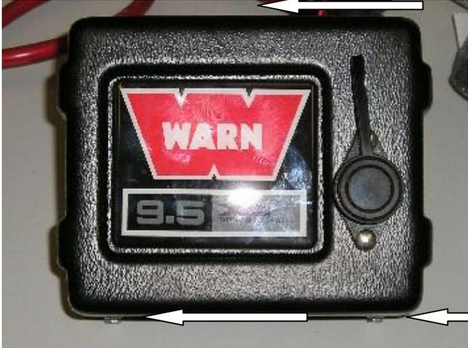
1. If fitting the **XP 9.5 winch**, remove the cover from the control box.
