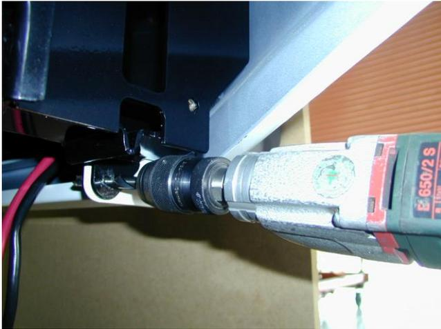
1. Next step is to lock pin the bar so there is no movement by drilling a 10mm hole on both sides of vehicle, fasten with 10mm x 25mm bolts plus 10mm hardware.
