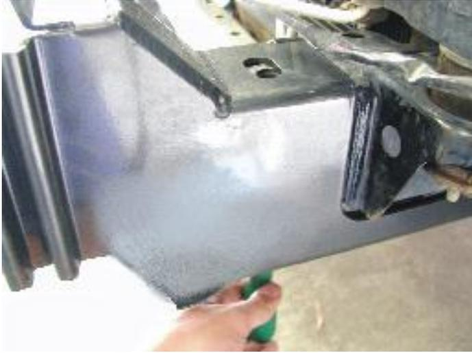
1. Using a long screwdriver insert it through the bottom hole so it passes through the tube packer. This may require a visual check from under the vehicle to see the position of the tube.
