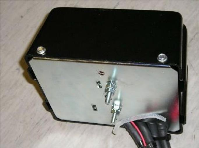
1. Replace the 2 cap screws, washers and nuts removed in step 17 above into original holes.
