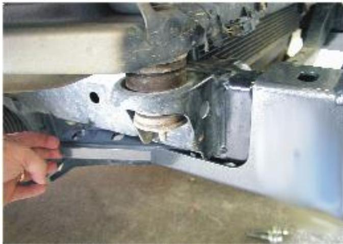
1. Slide the mount assy. over the chassis rails. Try not to shake the vehicle too severely as the tube packers may fall out of place.
