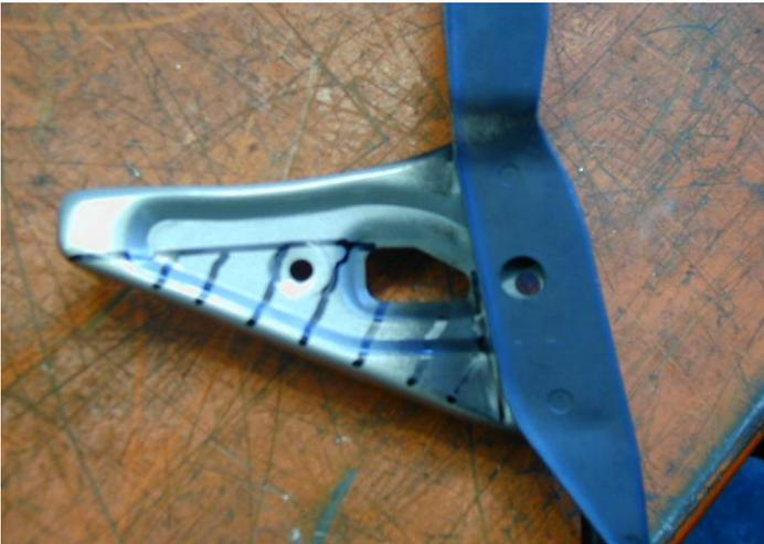
1. Once removed hold the upright in a vice and cut out the section shown with a hacksaw.
