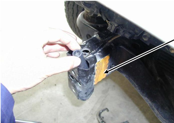
1. Insert the tube packers, one in each chassis arm. Line the bottom of the tube to the bottom hole of the chassis rail. Rest the top of the tube to the front of the chassis rail. The tube should be angled forward.
