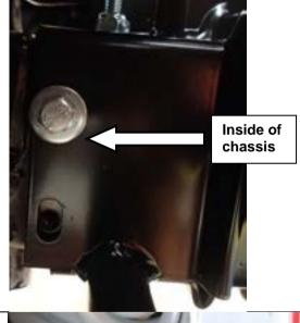
49. Align the mounting holes and fit two M12 x 170mm PC11.9 (2016+ single cab variants) or M12 x 140mm PC8.8 bolts with M12 flat washers through the chassis from the bottom. Fix with M12 flat washers, and nyloc nuts.
