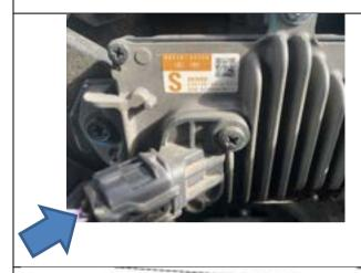
55. Connect radar extension loom to radar module.
