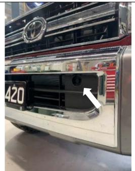
Remove two bumper cover retaining bolts. One on each side of the vehicle.
