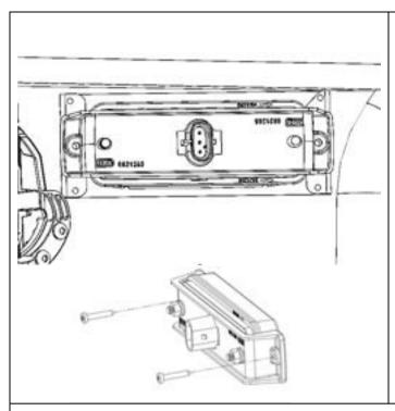
28. Install LED lamp with bracket into bull bar using 2 x 15mm mounting screws provided. (RH Shown).
