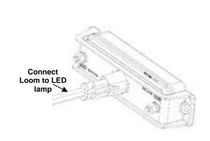
54. Connect indicator/clearance lights to the looms fitted in step 20.
