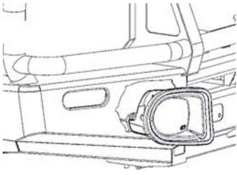
Fit fog lamp housings (3163082) into the bull bar fog lamp cut outs as shown. (RH Shown). Refer to fitting instructions (3789190) supplied in foglamp housing kit (3163082).
