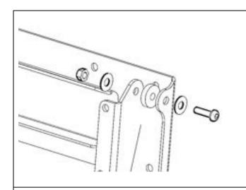
45. Fit number plate bracket to mount brackets using two M6x20mm screws, nyloc nuts, 16mm washers and nylon spacers provided.
