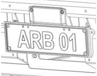
56. Fit number plate using four M6x12 Stainless Steel button head screws, four M6 flange nuts and four M6x12x1.2 Stainless Steel flat washers.
