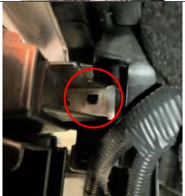
13. Remove the grille by unclipping retaining mechanism located at the inside bottom corner of the grille.
