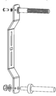
Mount each bracket onto the bed rack side panel using supplied fasteners.
